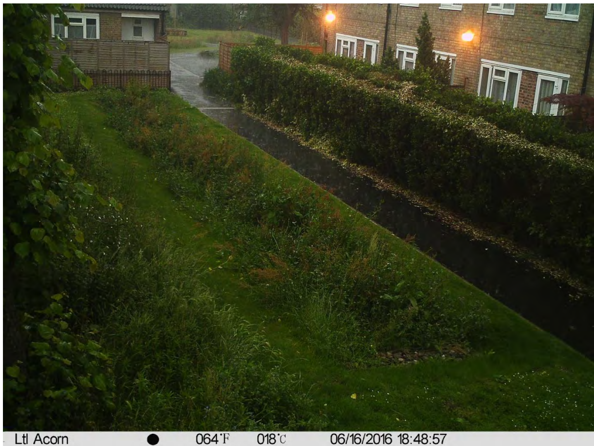
Figure 9. Time-lapse camera images from Alexandra House swale (FPC1). Image shows no evidence of swale filling excessively during period of highest rain intensity 18:30 to 20:00 on 16/06/2016 [32.8 mm of rain at maximum intensity of 188.8 mm/hr].
