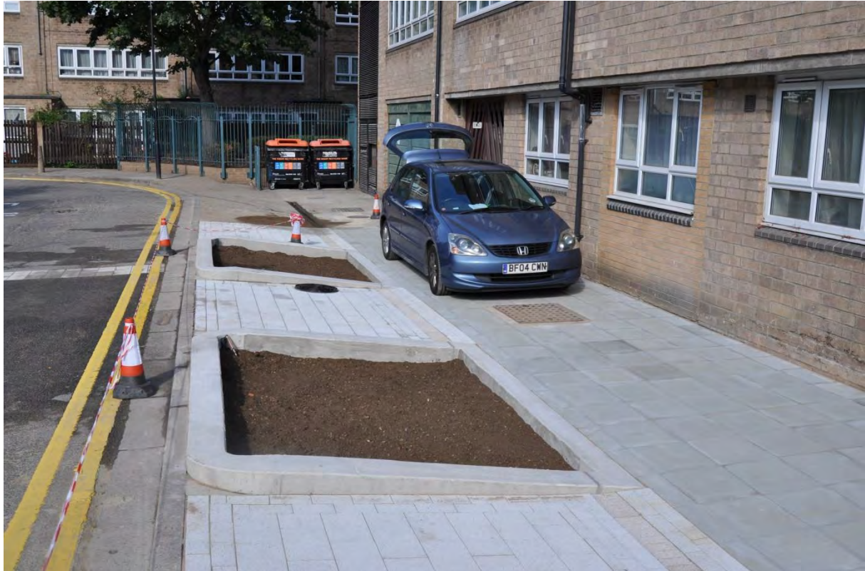
Figure 41. Image from the storm simulation event at the Sun Road rain gardens, Cheeseman Terrace Estate, 23rd September 2016. Image shows the rain gardens after the end of the stormwater simulation test with no signs of water pooling on any of the rain gardens.
