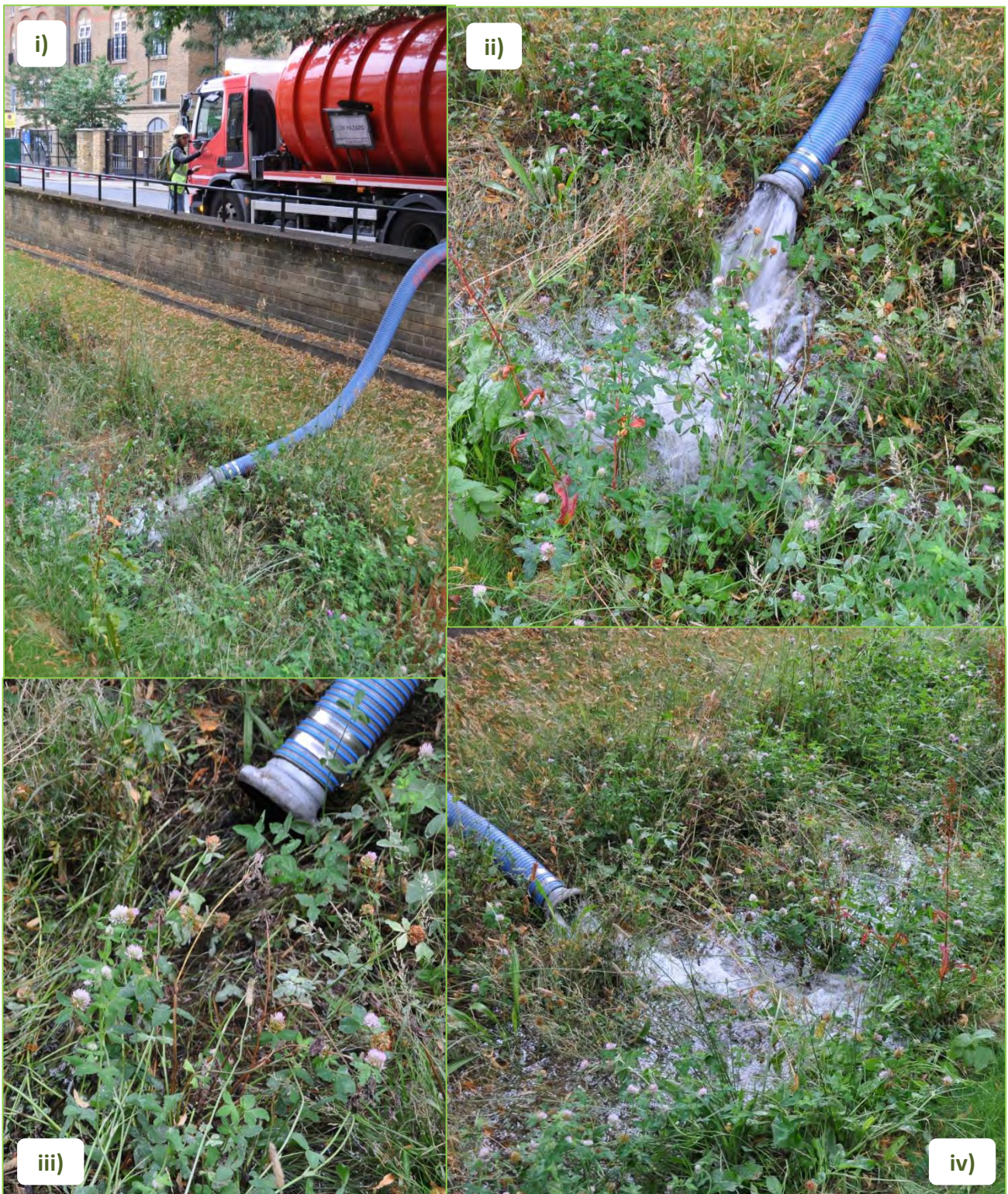
Figure 32. Images from the storm simulation event at Beatrice House swale, Queen Caroline Estate, 29th July 2016. Images show i) water release from tanker being timed to release 1000 Litres every six minutes; ii) 1000 Litres entering the centre of the swale; iii) condition of the swale after the first 1000 Litres; iv) condition of the swale as it starts to fill after several 1000 Litres releases.
