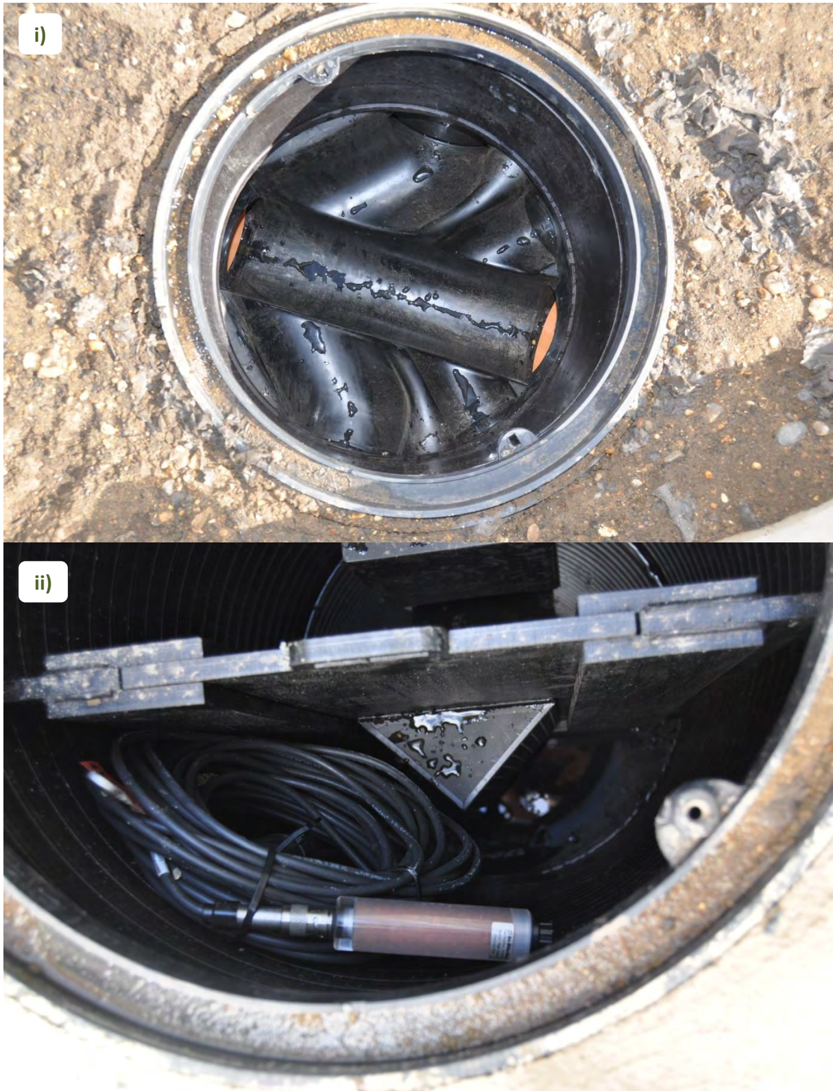
Figure 40. Images from the storm simulation event at the Sun Road rain gardens, Cheeseman Terrace Estate, 23rd September 2016. Images show i) the rain garden inspection chamber 30 minutes after the last of the 6,000 Litres of water was released and ii) the control flow chamber showing no release of water from the rain gardens following the 1 in 5 year storm event simulation.
