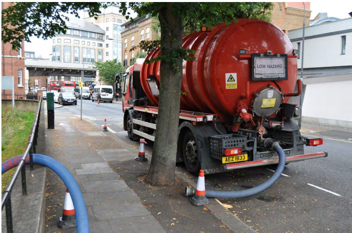
Figure 30. Water tanker delivering 10,000 Litres of non-potable water for the storm simulation event at Beatrice House swale. Storm simulation was carried out over the course of an hour on the 29th July 2016.
