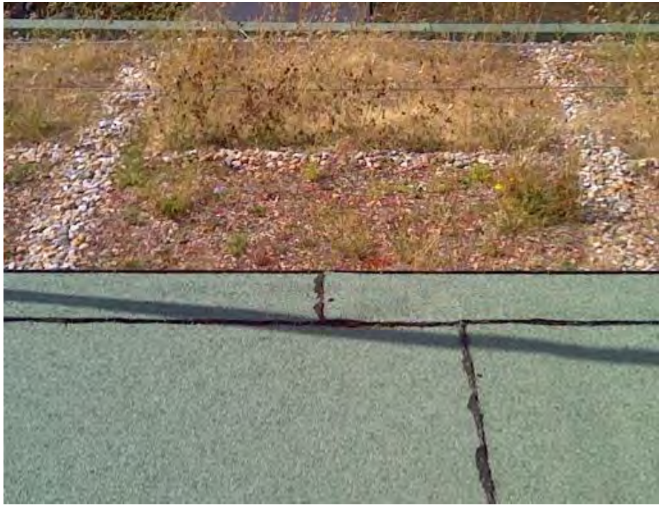
Figure 57. Photo and infrared image of green roof and neighbouring standard roof on Richard Knight House 27th July 2016. Infrared image reveals a temperature difference of 19.1 °C between the hottest and coolest areas within the field of view. A FLIR QuickReport spotmeter was used to identify individual temperatures within the field of view. Hottest temperatures (>33 °C) were associated with the non-greened areas of the flat roof. These areas were recorded as being hotter than the maximum daily temperature recorded by the nearby weather station (24.3 °C). Temperatures on sparsely vegetated areas of the greened roof were slightly lower than the non-greened roof area (31.6 to 32.7 °C). The coolest areas were associated with the vegetated areas of the green roof (24.9 to 26.4 °C).
