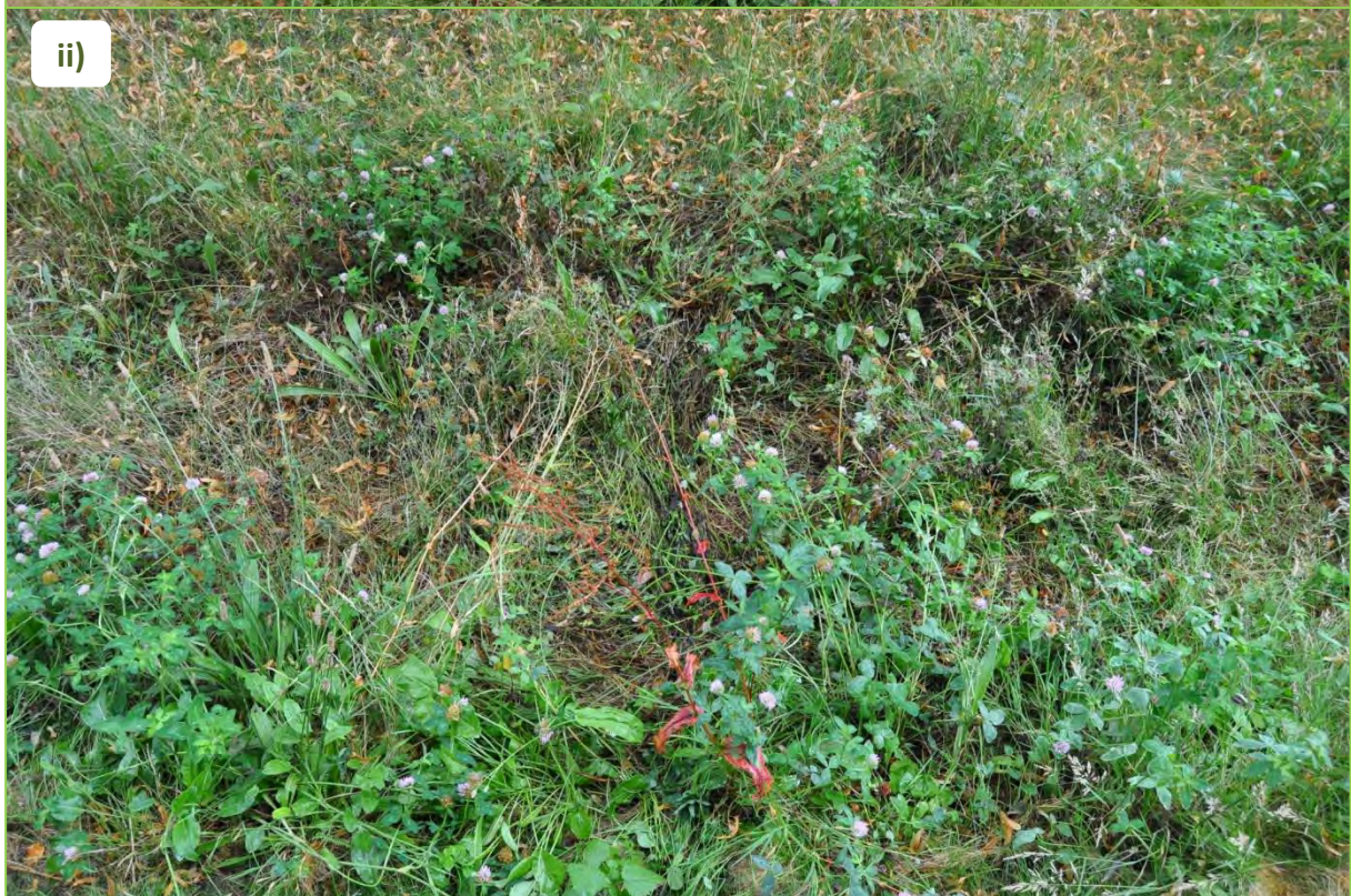
Figure 34. Images from the storm simulation event at Beatrice House swale, Queen Caroline Estate, 29th July 2016. Images show i) the Beatrice House swale immediately after the last of the 10,000 Litres of water was released and ii) the centre of the swale where the water was pumped in 15 minutes after the last of the water was released.
