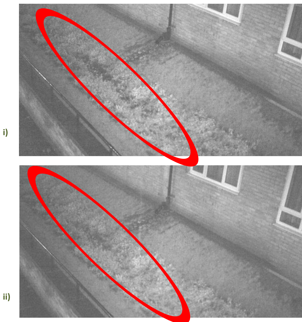
Figure 22. Time-lapse camera images from Beatrice House swale (FPC4). Images show i) evidence of swale filling during period of highest rain intensity 2am to 2:30am on 11/01/2016 [3.6 mm of rain at maximum intensity of 57.6 mm/hr] and ii) evidence of infiltration/conveyance by the time of the next time-lapse photo (~15 minutes later).
