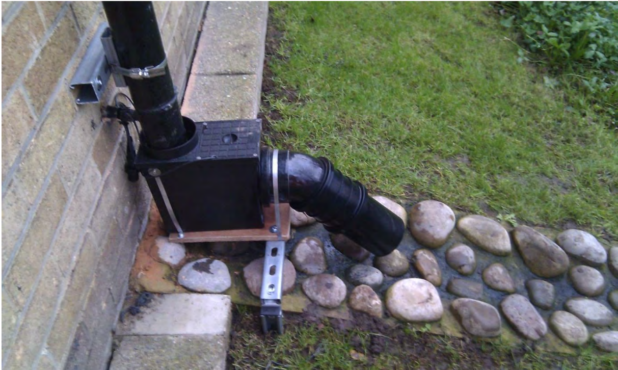
Figure 15. V-notch and levellogger installed at Beatrice House, Queen Caroline Estate, London Borough of Hammersmith & Fulham.
